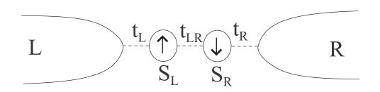
2 gated semi-conductor quantum dots in series between 2 leads
