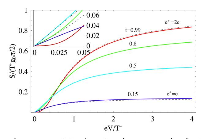
Close to critical point (K≈K<sub>c,</sub> t≈1) e\*=2e gives good fit except at very small V
