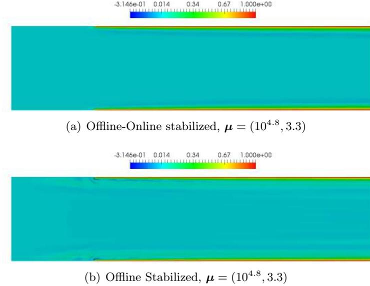
Figure 2.12: RB solution, stabilized Offline-Online and Offline,  $\boldsymbol{\mu} = (10^{4.8}, 3.3)$
