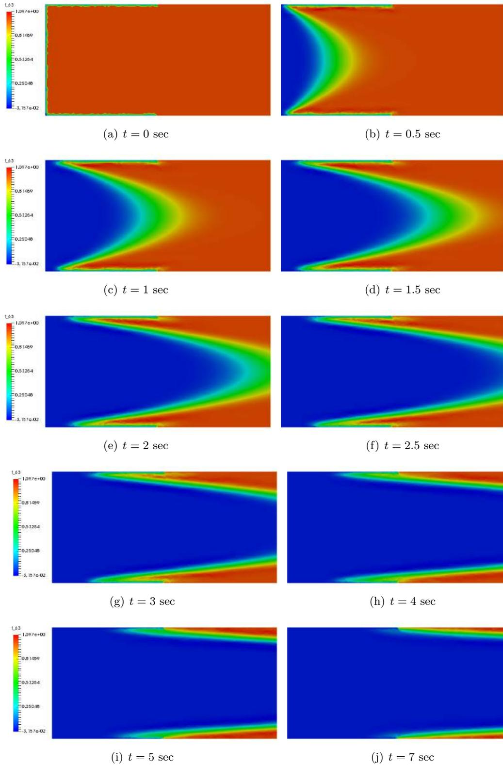
Figure 3.2: Plot of FE solution for parabolic Graetz problem at different times at  $\mu_1 = 1$  and  $\mu_2 = 1 \cdot 10^4$
