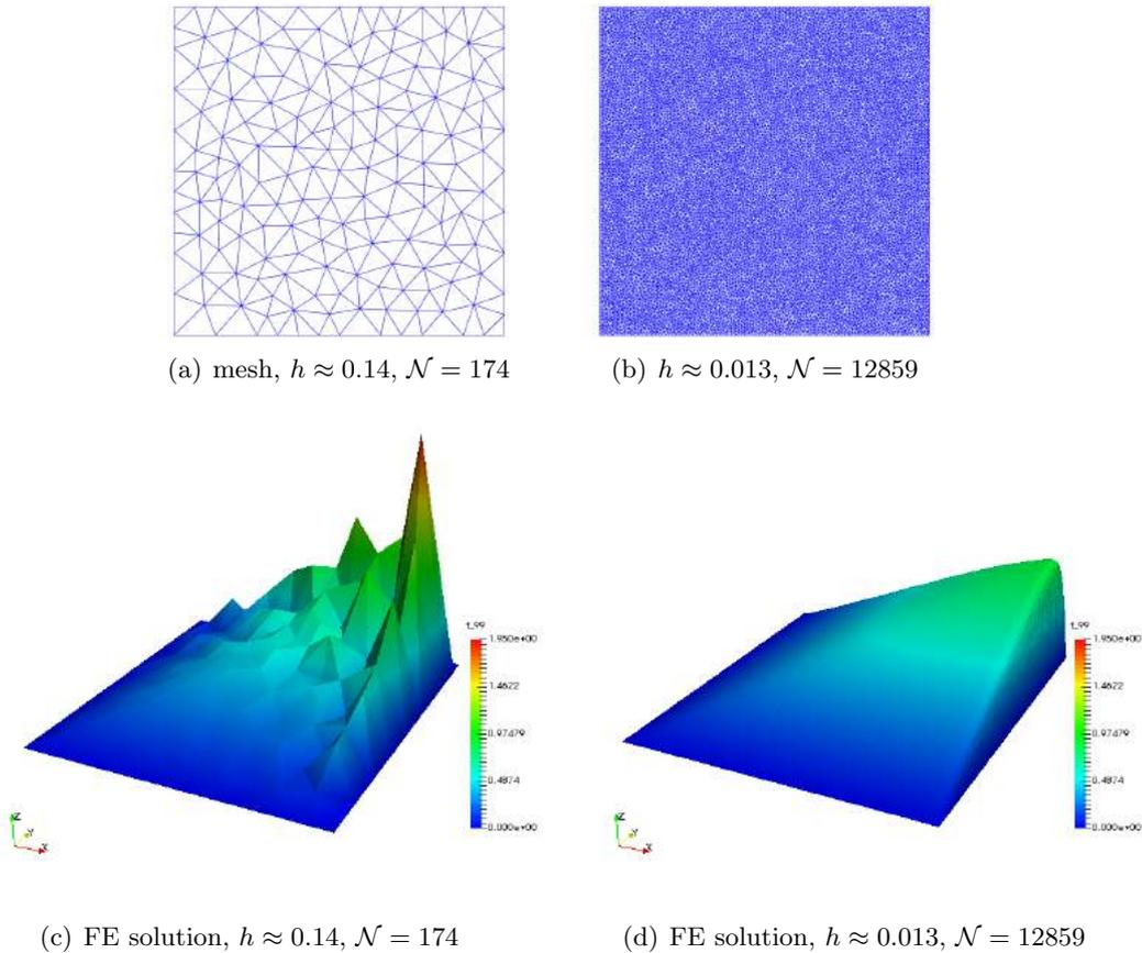
Figure 2.3: Two dimensional case, different mesh sizes
