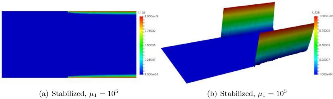
Figure 2.11: Stabilized SUPG, FE solution,  $\mu_1 = 10^5$
