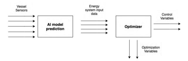
The framework manages the operations of an hybrid energy system such that fuel consumptions and emissions are minimized. We can identify two main parts in this project:
