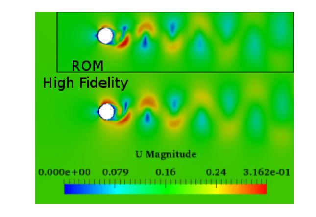
Comparison between velocity fields at Re=6000 with 20 modes. At the top is the reduced basis case lower at the bottom is the high fidelity one.
