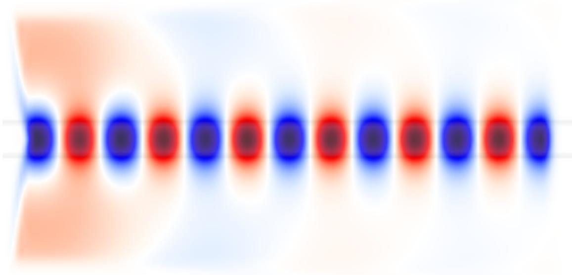
Figure 5: MEEP Waveguide propagation, src on the left
