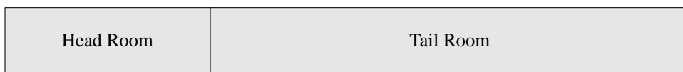
Figure 26 tcp_alloc_skb allocates additional space sufficient for headers, and reserves it as headroom
