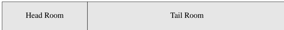
Figure 28 these functions allocate and reserve as headroom 16 bytes for the link header
