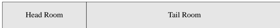
Figure 27 the IP fragmentation code allocates additional space for the current IP header and the link header, and reserves as headroom the space for the link header
