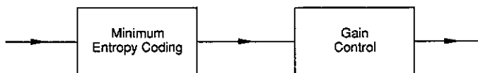
Figure 2. The problem is how to represent correlated signals most efficiently if the output neurons possess limited dynamic range. The simplest solution is shown as a two-stage process in this figure. In the first stage input signals are decorrelated to provide a minimum entropy code which can be followed by a simple cumulative probability map that functions as the gain control. The latter serves to fit the decorrelated signals into the limited dynamic range of each neuron independently.
