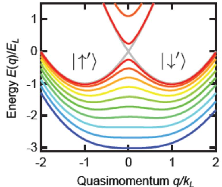
$$h_0 = \frac{1}{2} [(p_x - k_0 \sigma_z)^2 + p_{\perp}^2] + \frac{1}{2} \Omega \sigma_x + \frac{1}{2} \delta \sigma_z + V_{ext}$$
