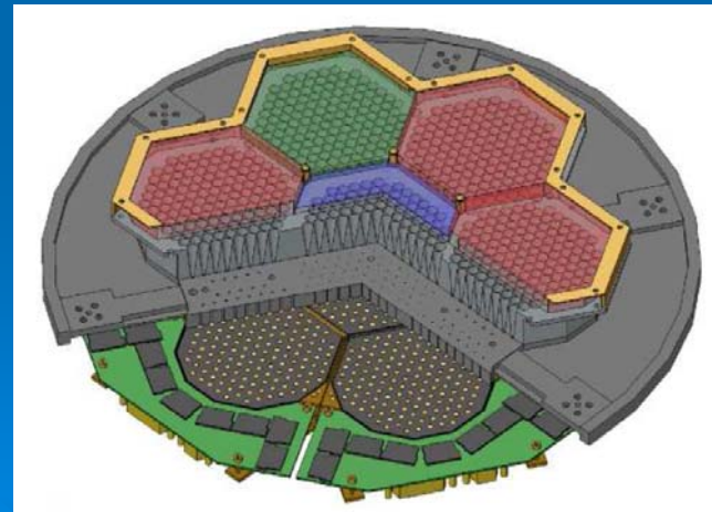
EBEx focal plane, courtesy of the EBEx collaboration
