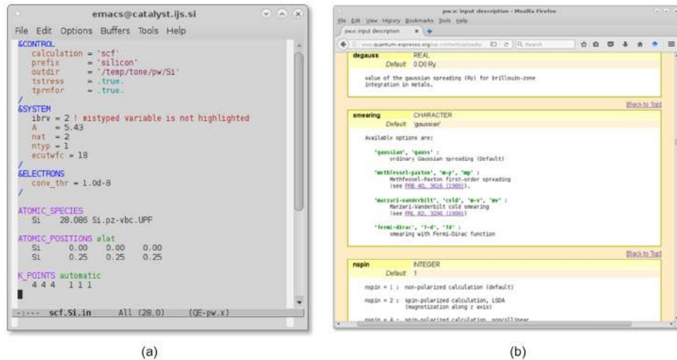
Figure 5. (a) pw.x input file opened in Emacs with pw-mode highlighting the following elements: namelists and their variables (blue and brown), cards and their options (purple and green), comments (red), string and logical variable values (burgundy and cyan, respectively). A mistyped variable (i.e. ibrv instead of ibrav ) is not highlighted. (b) An excerpt from the INPUT_PW.html file, which describes the pw.x input file syntax. Both the QE-emacs-modes and the INPUT_PW.html are automatically generated from the QUANTUM ESPRESSO's internal definition of the input file syntax.
