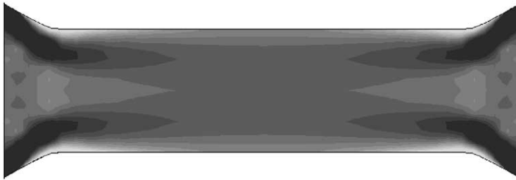
Fig. 5. Density plot of the von Mises stress at stretch s = 1.38 . For greater clarity, the full sample is displayed here (computations have been performed on one-quarter only).
