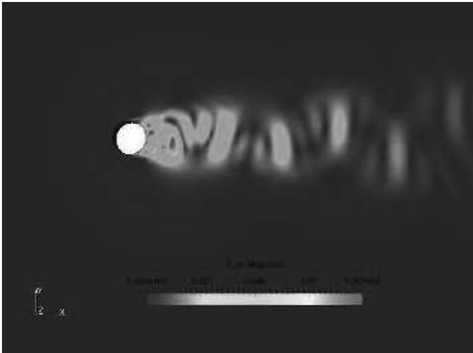
(B) The error difference between HF and ROM velocity for the case of a fixed cylinder immersed in flow at Re=6000 at time=82
